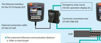
The maximum connection distance between the connector conversion box and the GOT is 10m.
