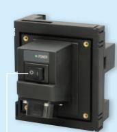
The power switch disables the GOT's emergency stop switch so that the cable and GOT can be disconnected without tripping the emergency stop signal.
