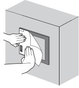
3) For attaching the protective sheet, make sure to fit the sheet on the GOT without wrinkles or air between the sheet and the GOT.
