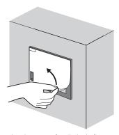
2) Remove the release paper from the back of a new protective sheet. Do not remove the protective film. Attach the protective sheet so that the sheet does not overlap with the USB environmental protection cover on the GOT.
