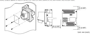
4.2 Mounting on the panel face (When installing the Connector Conversion Box on the panel surface)
