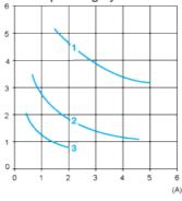
**DC-** Control of resistive loads and isolated solid state loads via optocoupler ( $L/R \le 1 \text{ ms}$ )
