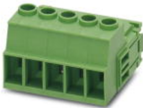
Plug component, Nominal current: 41 A, Rated voltage (III/2): 1000 V, Number of positions: 2, Pitch: 7.62 mm, Connection method: Screw connection, Color: green, Contact surface: Tin
