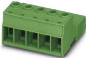
Plug component, Nominal current: 76 A, Rated voltage (III/2): 1000 V, Number of positions: 2, Pitch: 10.16 mm, Connection method: Screw connection, Color: green, Contact surface: Silver
