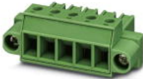
Plug component, Nominal current: 20 A, Rated voltage (III/2): 630 V, Number of positions: 3, Pitch: 7.62 mm, Connection method: Screw connection, Color: green, Contact surface: Tin
