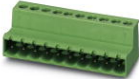
Plug component, Nominal current: 12 A, Rated voltage (III/2): 320 V, Number of positions: 8, Pitch: 5.08 mm, Connection method: Screw connection, Color: green, Contact surface: Tin
