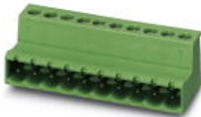
Plug component, Nominal current: 12 A, Rated voltage (III/2): 320 V, Number of positions: 4, Pitch: 5.08 mm, Connection method: Screw connection, Color: green, Contact surface: Tin
