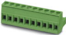
Plug component, Nominal current: 12 A, Rated voltage (III/2): 320 V, Number of positions: 9, Pitch: 5.08 mm, Connection method: Screw connection, Color: green, Contact surface: Tin
