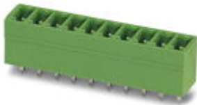
Header, Nominal current: 8 A, Rated voltage (III/2): 160 V, Number of positions: 10, Pitch: 3.81 mm, Color: green, Contact surface: Tin, Assembly: Soldering
