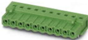
Header, Nominal current: 12 A, Rated voltage (III/2): 320 V, Number of positions: 8, Pitch: 5.08 mm, Color: green, Contact surface: Tin, Assembly: Soldering
