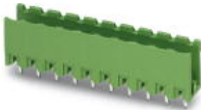
Header, Nominal current: 12 A, Rated voltage (III/2): 320 V, Number of positions: 8, Pitch: 5 mm, Color: green, Contact surface: Tin, Assembly: Soldering
