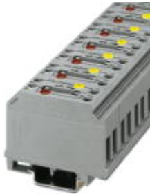
Ground disconnect terminal block with screw connection, voltage 110 - 250 V AC/DC, current: 0.5 - 1 mA, cross section: 0.5 - 6 mm 2 , width: 22.5 mm, color: gray
