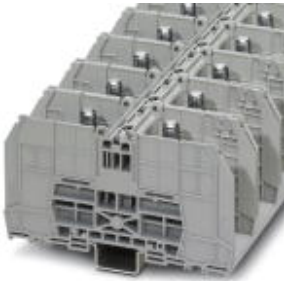
Bolt connection terminal block, Connection method: Bolt connection, Number of positions: 1, Cross section: 6 mm 2 - 150 mm 2 , AWG: 10 - 300, Width: 41 mm, Color: gray, Mounting type: NS 35/7,5, NS 35/15
