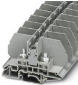
Bolt connection terminal block, Connection method: Bolt connection, Cross section: 2.5 mm 2 - 35 mm 2 , AWG: 12 - 2, Width: 17 mm, Height: 48.6 mm, Color: gray, Mounting type: NS 35/7,5, NS 35/15, NS 32
