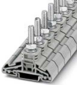
High Current Connectors, Connection method: Bolt connection, Cross section: 2.5 mm 2 - 50 mm 2 , AWG: 14 - 1/0, Width: 21 mm, Height: 63.5 mm, Color: gray, Mounting type: NS 35/7,5, NS 35/15
