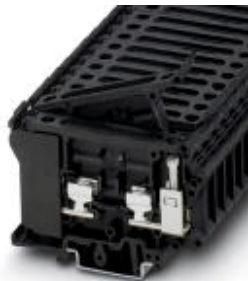
Fuse terminal block for cartridge fuse insert, cross section: 0.5 - 16 mm 2 , AWG: 26 - 8, width: 10.2 mm, color: black
