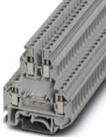
Double-level terminal block, Cross section: 0.2 mm 2 - 4 mm 2 , AWG: 24 - 12, Connection type: Screw connection, Width: 6.2 mm, Color: gray, Mounting type: NS 35/7,5, NS 35/15, NS 32
