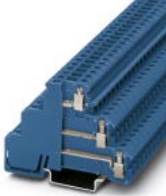
Sensor/actuator terminal block, Cross section: 0.2 mm 2 - 4 mm 2 , AWG: 24 - 12, Connection type: Screw connection, Width: 6.2 mm, Color: blue, Mounting type: NS 35/7,5, NS 35/15
