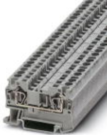
Feed-through terminal block, Connection method: Spring-cage connection, Cross section: 0.08 mm 2 - 6 mm 2 , AWG: 28 - 10, Width: 6.2 mm, Color: red, Mounting type: NS 35/7,5, NS 35/15
