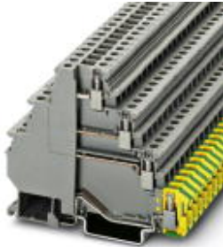
Protective conductor double-level terminal block, Cross section: 0.2 mm 2 - 4 mm 2 , AWG: 24 - 12, Connection type: Screw connection, Width: 6.2 mm, Color: gray, Mounting type: NS 35/7,5, NS 35/15
