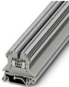
Feed-through terminal block, Connection method: Screw connection, Cross section: 0.14 mm 2 - 1.5 mm 2 , AWG: 26 - 16, Width: 4.2 mm, Color: gray, Mounting type: NS 35/7,5, NS 35/15, NS 32
