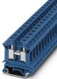
Feed-through terminal block, Connection method: Screw connection, Cross section: 0.5 mm 2 - 16 mm 2 , AWG: 20 - 6, Width: 10.2 mm, Color: blue, Mounting type: NS 35/7,5, NS 35/15, NS 32
