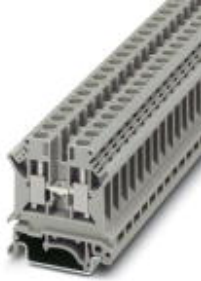
Feed-through terminal block, Connection method: Screw connection, Cross section: 0.2 mm 2 - 10 mm 2 , AWG: 24 - 8, Width: 8.2 mm, Color: gray, Mounting type: NS 35/7,5, NS 35/15, NS 32
