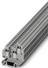
Micro terminal, Cross section: 0.14 mm 2 - 1.5 mm 2 , AWG: 26 - 16, Connection type: Screw connection, Width: 4.2 mm, Color: gray, Mounting type: NS 15
