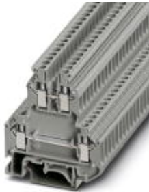
Double-level terminal block, Cross section: 0.2 mm 2 - 4 mm 2 , AWG: 24 - 12, Connection type: Screw connection, Width: 5.2 mm, Color: gray, Mounting type: NS 35/7,5, NS 35/15, NS 32
