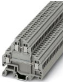
Micro terminal, Cross section: 0.14 mm 2 - 1.5 mm 2 , AWG: 26 - 16, Connection type: Screw connection, Width: 4.2 mm, Color: gray, Mounting type: NS 15, NS 35/7,5, NS 35/15
