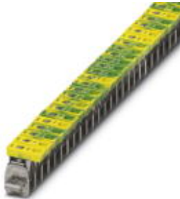
Connection terminal block, Connection method Screw connection, Load current : 76 A, Cross section: 1.5 mm 2 - 16 mm 2 , Width: 9.8 mm, Color: green-yellow
