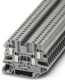
Feed-through terminal block, Connection method: Screw connection, Cross section: 0.14 mm 2 - 6 mm 2 , AWG: 26 - 10, Width: 6.2 mm, Color: gray, Mounting type: NS 35/7,5, NS 35/15
