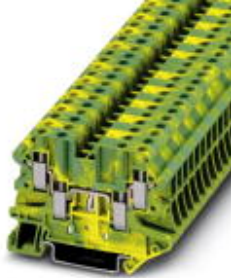
Ground modular terminal block, Connection method: Screw connection, Cross section: 0.14 mm 2 - 6 mm 2 , AWG: 26 - 10, Width: 6.2 mm, Color: green-yellow, Mounting type: NS 35/7,5, NS 35/15
