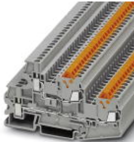
Feed-through terminal block, Connection method: Quick connection, Screw connection, Cross section: 0.25 mm 2 - 1.5 mm 2 , Width: 5.2 mm, Color: gray, Mounting: NS 35/7,5, NS 35/15
