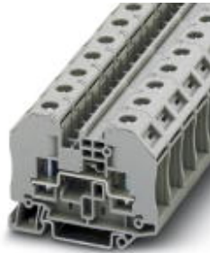
Feed-through terminal block with bolt connection, cross section: 0.1 - 6 mm 2 , AWG: 26 - 10, width 16.3 mm, color: Gray
