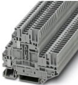
Double-level terminal block, Cross section: 0.14 mm 2 - 4 mm 2 , AWG: 26 - 12, Connection type: Screw/plug-in connection, Width: 5.2 mm, Color: gray, Mounting type: NS 35/7,5, NS 35/15
