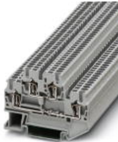
Double-level spring-cage terminal block, Cross section: 0.08 mm 2 - 1.5 mm 2 , AWG: 28 - 16, Connection type: Spring-cage connection, Width: 4.2 mm, Color: gray, Mounting type: NS 35/7,5, NS 35/15
