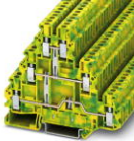
Ground modular terminal block, Cross section: 0.14 mm 2 - 4 mm 2 , AWG: 26 - 12, Connection type: Screw connection, Width: 5.2 mm, Color: green/yellow, Mounting type: NS 35/7,5, NS 35/15
