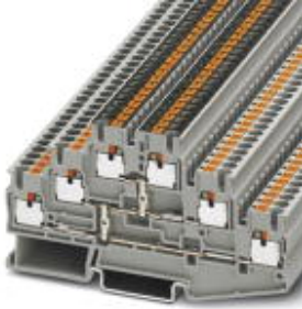
Multi-level terminal block, Connection method: Push-in connection, Cross section: 0.14 mm 2 - 4 mm 2 , AWG: 26 - 12, Width: 5.2 mm, Color: gray, Mounting type: NS 35/7,5, NS 35/15
