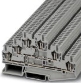
Multi-level terminal block, Connection method: Spring-cage connection, Cross section: 0.08 mm 2 - 4 mm 2 , AWG: 28 - 12, Width: 5.2 mm, Color: gray, Mounting type: NS 35/7,5, NS 35/15
