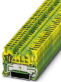
Spring cage ground terminal block, Connection method: Spring-cage/plug-in connection, Cross section: 0.08 mm 2 - 4 mm 2 , AWG: 28 - 12, Width: 5.2 mm, Color: green-yellow, Mounting type: NS 35/7,5, NS 35/15
