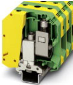
Ground modular terminal block, Connection method: Screw connection, Cross section: 25 mm 2 - 95 mm 2 , AWG: 4 - 3/0, Width: 25 mm, Color: green-yellow, Mounting type: NS 35/7,5, NS 35/15, NS 32
