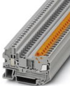
Feed-through terminal block, Connection type: Quick connection, Screw connection, Cross section: 0.5 mm 2 - 2.5 mm 2 , AWG :20- 14, Width: 6.2 mm, Color: gray, Mounting: NS 35/7,5, NS 35/15
