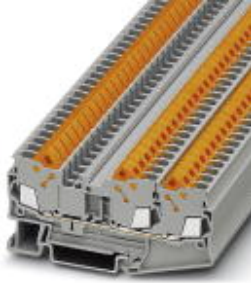
Feed-through terminal block, Connection method: Quick connection, Cross section: 0.5 mm 2 - 2.5 mm 2 , AWG: 20 - 14, Width: 6.2 mm, Height: 37.8 mm, Color: gray, Mounting type: NS 35/7,5, NS 35/7,5
