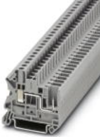
Feed-through terminal block, Connection method: Screw/plug-in connection, Cross section: 0.14 mm 2 - 6 mm 2 , AWG: 26 - 10, Width: 6.2 mm, Color: gray, Mounting type: NS 35/7,5, NS 35/15
