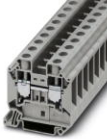
Feed-through terminal block, Connection method: Screw connection, Cross section: 1.5 mm 2 - 25 mm 2 , AWG: 16 - 4, Width: 12.2 mm, Height: 54.4 mm, Color: gray, Mounting type: NS 35/7,5, NS 35/15
