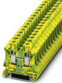
Ground modular terminal block, Connection method: Screw connection, Cross section: 0.2 mm 2 - 10 mm 2 , AWG: 24 - 8, Width: 8.2 mm, Color: green-yellow, Mounting type: NS 35/7,5, NS 35/15
