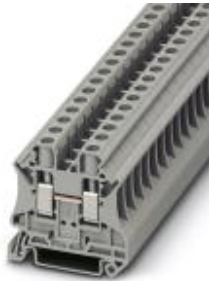
Feed-through terminal block, Connection method: Screw connection, Cross section: 0.2 mm 2 - 10 mm 2 , AWG: 24 - 8, Width: 8.2 mm, Color: gray, Mounting type: NS 35/7,5, NS 35/15
