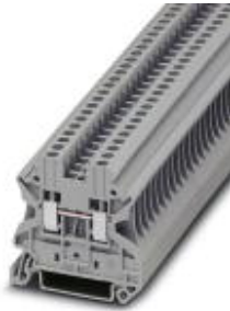
Feed-through terminal block, Connection method: Screw connection, Cross section: 0.14 mm 2 - 4 mm 2 , AWG: 26 - 12, Width: 5.2 mm, Color: gray, Mounting type: NS 35/7,5, NS 35/15
