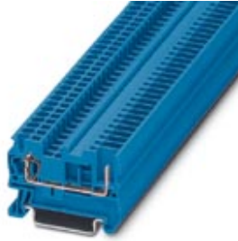
Feed-through terminal block, Connection method: Spring-cage/plug-in connection, Cross section: 0.08 mm 2 - 4 mm 2 , AWG: 28 - 12, Width: 5.2 mm, Color: blue, Mounting type: NS 35/7,5, NS 35/15
