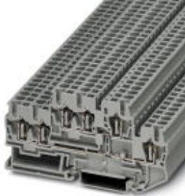
Double-level spring-cage terminal block, Cross section: 0.08 mm 2 - 4 mm 2 , AWG: 28 - 12, Connection type: Spring-cage connection, Width: 5.2 mm, Color: gray, Mounting type: NS 35/7,5, NS 35/15
