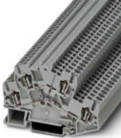
Double-level spring-cage terminal block, Cross section: 0.08 mm 2 - 4 mm 2 , AWG: 28 - 12, Connection type: Spring-cage connection, Width: 5.2 mm, Color: gray, Mounting type: NS 35/7,5, NS 35/15
